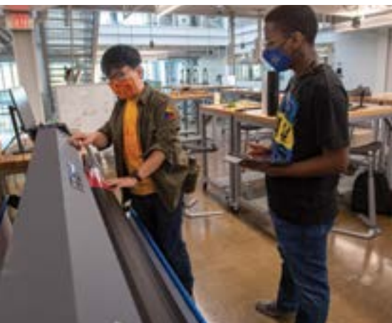
DI Fellows Program students Ray Yang and Khalil Thompson manage the 60-inch-wide vinyl cutter available in the PrintLab, one of seven DI Labs inside the DI Hub. The vinyl cutter allows users to create super-wide cut vinyl graphics that can be applied to hard and soft surfaces.
